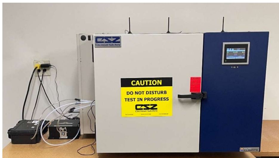
Figure A-1. An image of the chamber and sampling setup for the lab-based verification.
